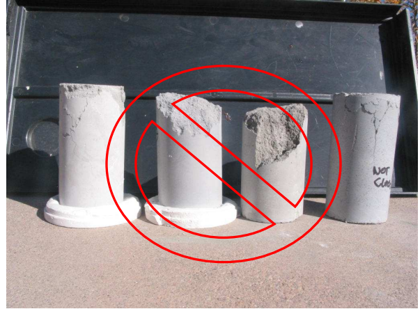
Figure 2: Incorrect cylinder breaks
